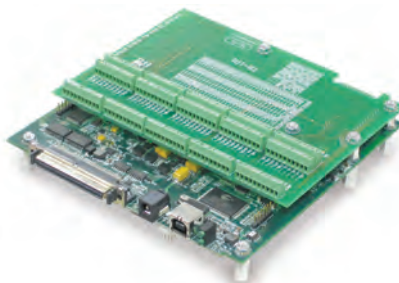
DaqBoard/3001USB with TB-101 screw-terminal board attached
