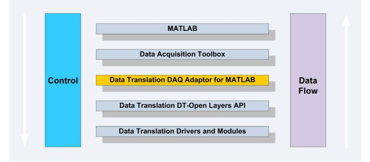
The above diagram depicts the hierarchy of control and data flow from MATLAB to Data Translation DT-Open Layers-compliant modules. The Data Translation DAQ Adaptor for MATLAB passes commands and data between the Data Acquisition Toolbox of MATLAB and the Data Translation hardware to provide a seamless, integrated programming environment.
