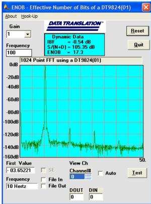
ENOB results are shown for input ranges at one-half full scale (-6 dB) and at full scale. The ENOBs are a small amount lower as the input range increases due to slew rate limitations on the amplifier at 18.3 bits and 17.2 bits. These are much higher than comparable solutions, giving greater accuracy and stability.
