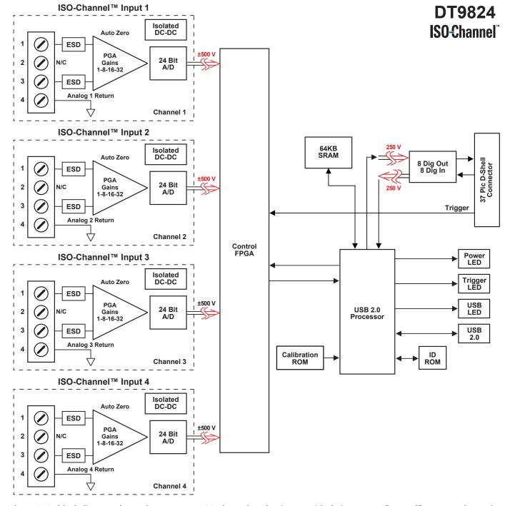
The DT9824 block diagram shows the 4 separate ISO-Channel analog inputs with their separate "ground" return paths. Each analog input has its own 24-bit sigma-delta A/D and auto-zero programmable gain amplifier (PGA) to achieve unprecedented stability and accuracy. CMRR is better than 150 dB, system gain error of better than ±0.003%, system zero error of less than ±50 uV, give accuracy and stability performance beyond any other solution.
