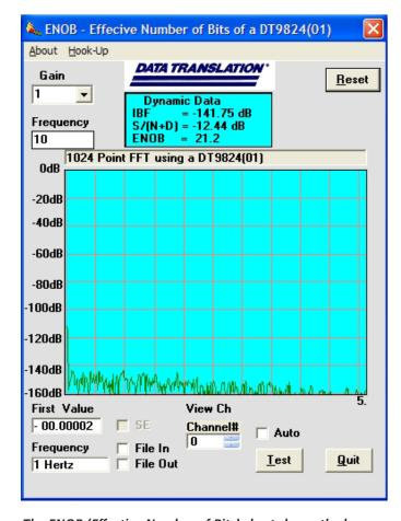
The ENOB (Effective Number of Bits) chart shows the low level of noise, baseline noise at better than 21 bits, with zero signal at the input (input shorted) that is generated at the output. ENOB chart is an FFT plot that points out harmonics and other error producing results. Other plots at various input ranges are shown on the following pages.
