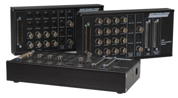
Portable measurements can now be made with 4, 8, or 16 individual A/D channels. Each 24-bit sigma-delta A/D runs in parallel to prevent interference between channels. The DT9826 is fully featured with DIO, 32-bit counter/timers, tachometer, and multi-trigger modes. Software options abound to accommodate any environment. Available in BNC box or as embedded board-level OEM version.
