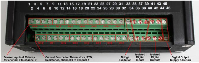
Input connections are easily made via screw terminals for all sensor inputs.
