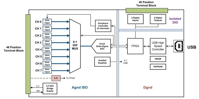
Block diagram of the DT9829 shows that up to 8 sensors of any type can be connected for precision measurement. Applications in industry, lab, or field can take advantage of the portable operation running off USB power.
