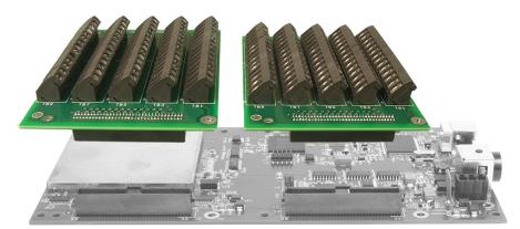
The EP355 screw terminal panel plugs into the J2 or J3 connector on the OEM version of the DT9844 module.
