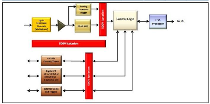
The block diagram of the DT9844 shows the  $\pm 500$  V isolation between three subsystems and the host computer. All circuitry is designed to preserve the lowest noise for analog data acquisition.
