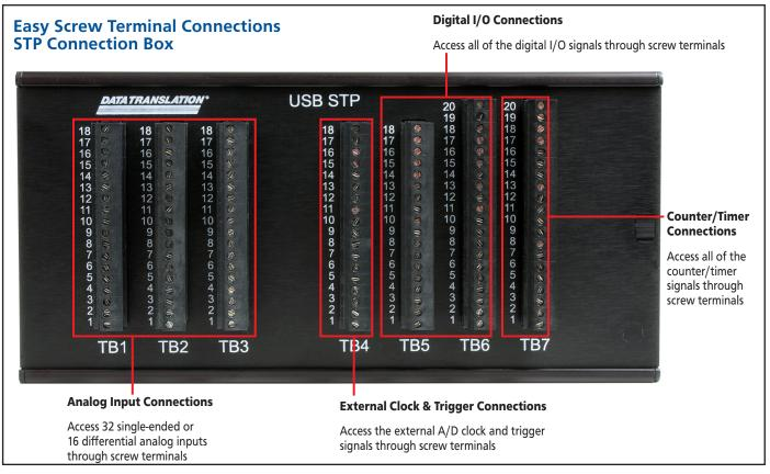
The STP connection box is available for easy signal connections on the 32-channel version of the module
