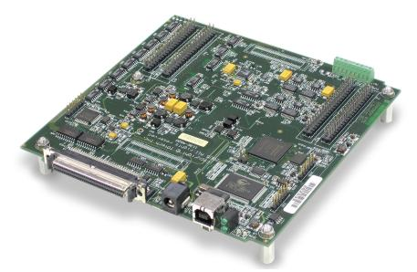
*The USB-2500 Series boards are high-Speed Multifunction DAQ Boards designed for OEM and embedded applications*
