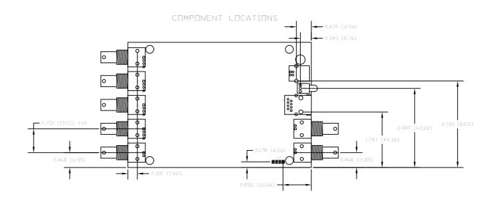
MAXIMUM COMPONENT HEIGHT COMPONENT SIDE = .528 [13.41 SOLDER SIDE = .100 [2.54]
