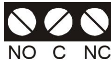
Figure 2. Typical relay channel
