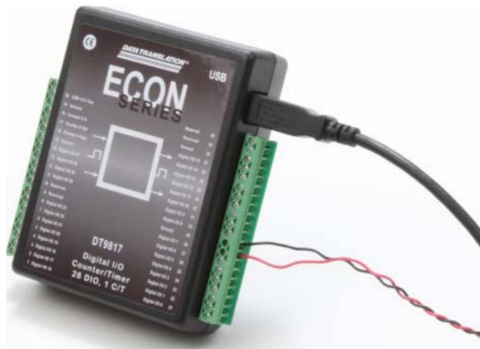
Figure 5: Wiring to the Screw Terminals of a Module
