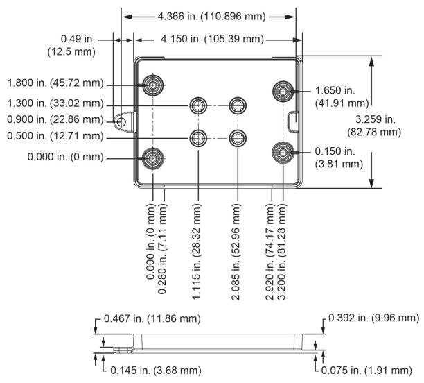
Figure 8. E-DIO24 bottom enclosure dimensions
