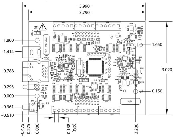
Figure 7. E-DIO24 device circuit board dimensions
