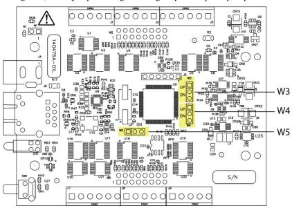
Figure 5. Pull-up/down jumper locations
