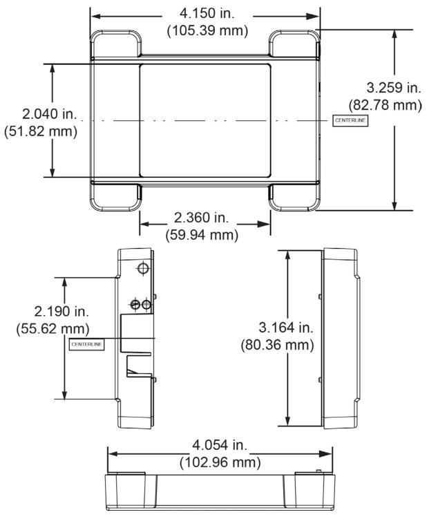
Figure 9. E-DIO24 top enclosure dimensions
