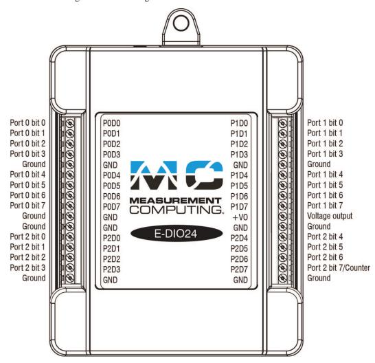
Figure 2. E-DIO24 pinout
