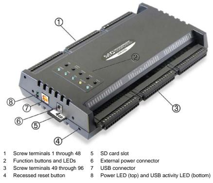
Figure 4. LGR-5320 Series external components
