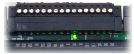
Figure 6. LGR-5320 Series screw terminals and LEDs
