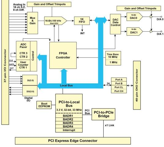
Figure 1. PCIe-DAS1602/16 functional block diagram
