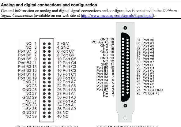
Figure 12. Digital I/O connector pin out
