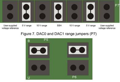
Figure 8. DAC0 (P5) and DAC1 (P6) unipolar/bipolar jumpers
