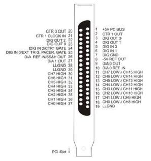
Figure 11. Main I/O connector pin out
