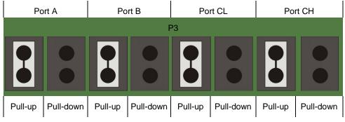
Figure 10. Pull-up/pull-down jumpers (P3)
