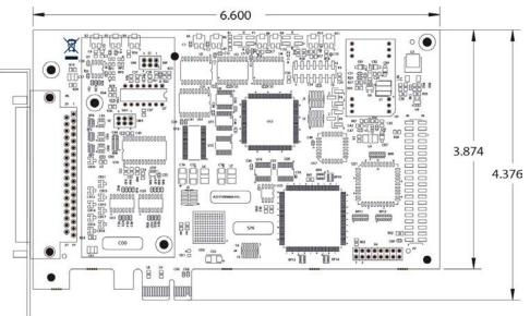
Figure 17. PCIe-DAS1602/16 circuit board dimensions (inches)
