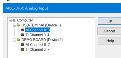
3. Double-click on the Analog Input module to open its dialog box.
