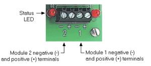
The screw terminal/module numbers correspond to 8255 ports:
