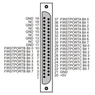
Do not make connections to pins marked "NC".
