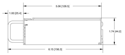
Figure 10. Enclosure dimensions – side
