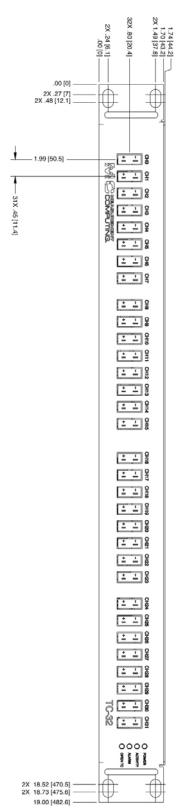
Figure 8. Enclosure dimensions - front
