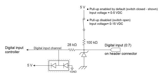
Figure 5. Digital input connection example
