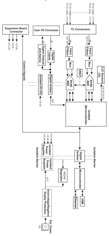
Figure 1. TC-32 functional block diagram
