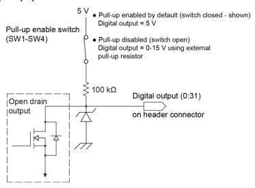
Figure 6. Digital output connection example
