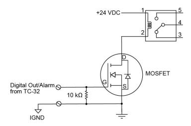
Figure 7. Example of digital output/alarm controlling a relay
