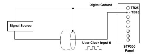
Figure 35: Connecting Frequency Measurement Signals without an External Gate Input (Shown for Clock Input 0)
