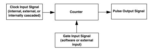
Figure 31: Counter/Timer Channel
