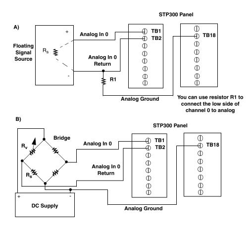
Figure 10: Connecting Differential Voltage Inputs (Shown for Channel 0)
