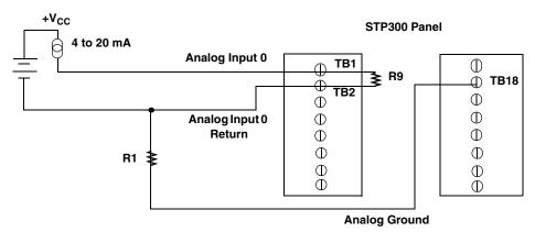
Use current shunt resistor R9 to convert current to voltage; 250  $\Omega$  for 4 to 20 mA = 1 to 5 V. The common-side of the external loop supply must either connect to analog ground or, if needed, to a bias return resistor (R1 in this case).
