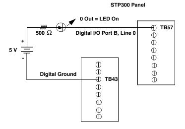
Figure 16: Connecting Digital Outputs (Shown for Channel 0, Port B)
