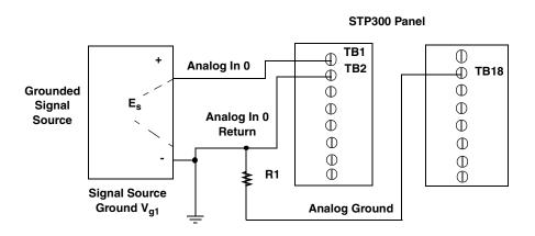
Resistor R1 should be installed for bias return in case the external ground is floating.
