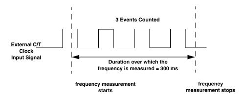
Figure 37: Example of Frequency Measurement
