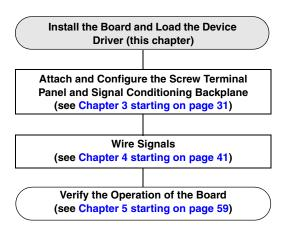
**Note:** All DT300 Series boards are factory-calibrated and require no further adjustment prior to installation. If you are using the DT300 Series board and decide later to recalibrate it, refer to Chapter 8 starting on page 117 for instructions.
