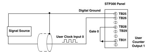
Figure 20: Connecting Frequency Measurement Signals (Shown for Clock Input 0 and External Gate 0)
