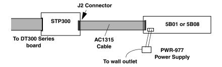
Figure 6: Connecting the 5B01 or 5B08 Backplane to the STP300
