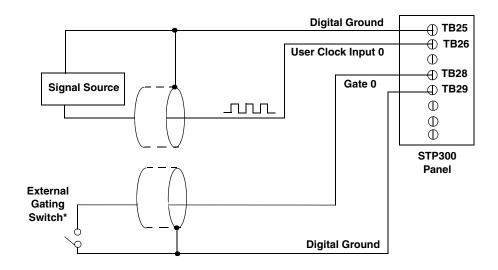
\*An internal 33 ohm series resistor is used.
