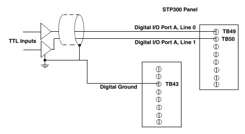
Figure 15: Connecting Digital Inputs (Shown for Channels 0 and 1, Port A)
