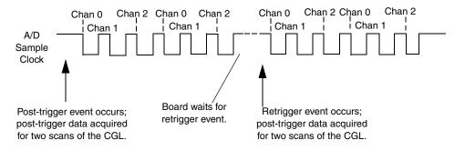
Figure 26: Continuous Post-Trigger Mode with Triggered Scan
