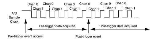
Figure 29: Continuous About-Trigger Mode
