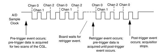
Figure 28: Continuous Pre-Trigger Mode with Triggered Scan
