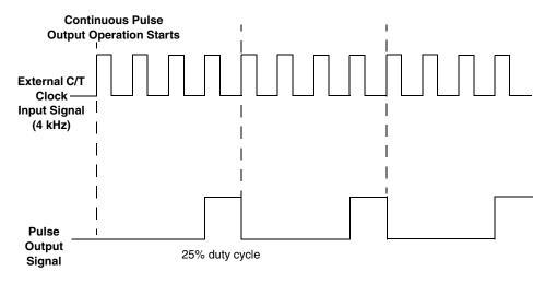
Figure 40: Example of Rate Generation Mode with a 25% Duty Cycle
