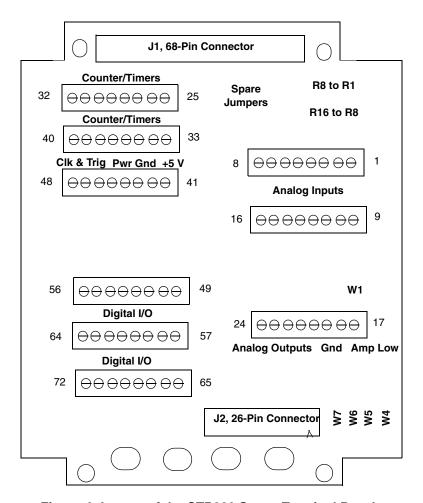
Figure 4: Layout of the STP300 Screw Terminal Panel
