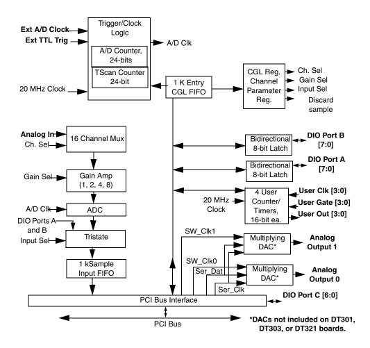
Figure 24: Block Diagram of the DT300 Series Boards
