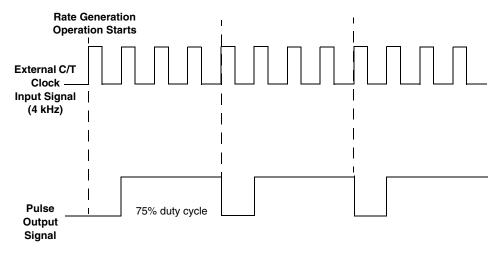
Figure 39: Example of Rate Generation Mode with a 75% Duty Cycle
