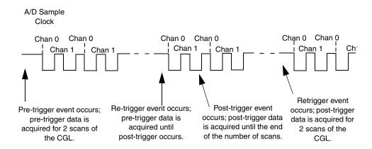
Figure 30: Continuous About-Trigger Mode with Triggered Scan
