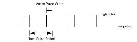
Figure 32: Example of a Low-to-High Pulse Output Type
