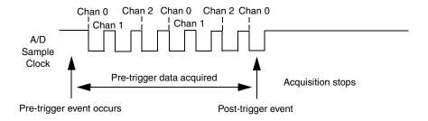
Figure 27: Continuous Pre-Trigger Mode
