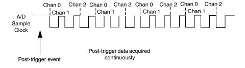
Figure 25: Continuous Post-Trigger Mode without Triggered Scan
