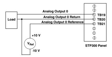
Figure 13: Connecting Analog Output Voltages Using an External +10 V Reference (Shown for Channel 0)
