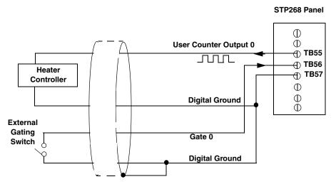
Figure 49, Figure 50, and Figure 51 show examples of connecting pulse output applications to the STP268 screw terminal panel. Other combinations of signals can be used.
