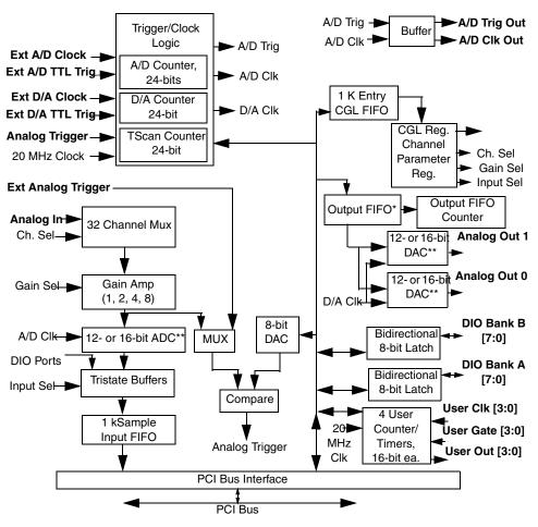
\*The DT3010, DT3010-268, and DT3016 have a 4 kSample output FIFO; the DT3010/32 and DT3010/32-268 have a 32 kSample output FIFO.\*\*Only the DT3016 has a 16-bit ADC and 16-bit DACs.
