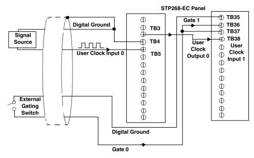
Note that you can internally cascade counters using software; if you internally cascade the counters, you do not have to make the external cascading connections. Note also that this example shows the use of an external gate; however, this connection is not required.
