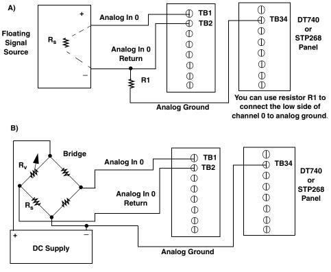
Note that the signals shown for the STP268 screw terminal panel correspond to connector J1.
