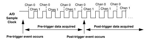
Figure 61: Continuous About-Trigger Mode
