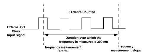
Figure 69: Example of Frequency Measurement
