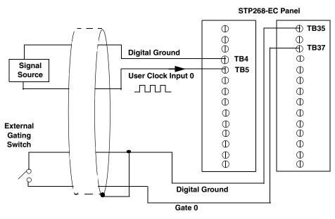
In this example, rising clock edges are counted while the gate is active.
