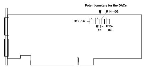
Figure 79: Location of Potentiometers R12 to R15 on the DT3016 Board
