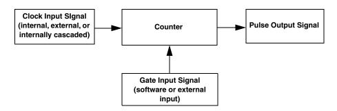
Figure 63: Counter/Timer Channel
