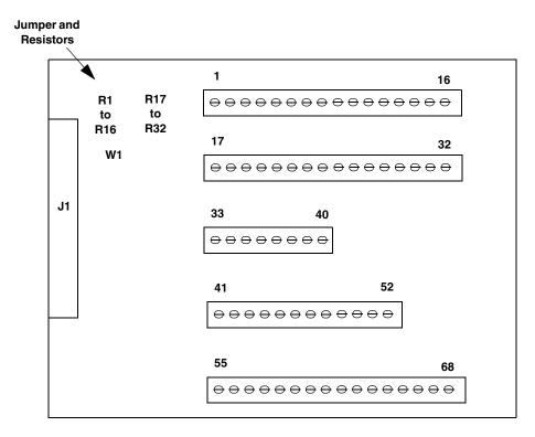
Figure 13: Layout of the STP268 Screw Terminal Panel
