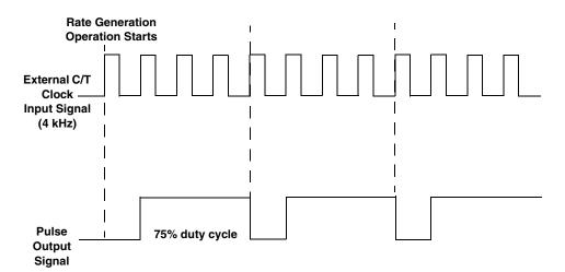
Figure 71: Example of Rate Generation Mode with a 75% Duty Cycle
