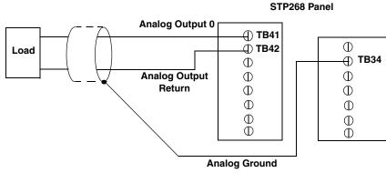
Note that the signals shown for the STP268 screw terminal panel correspond to connector J1.
