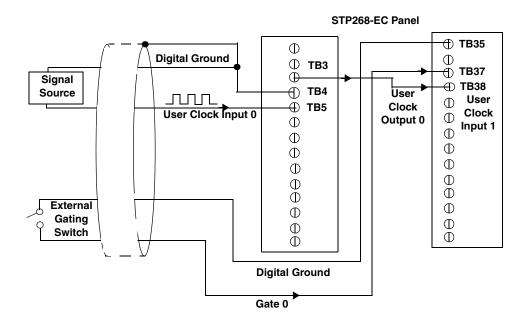
Figure 53: Cascading Counters to the STP268-EC (Shown for Rate Generation Using Counters 0 and 1 and External Gate 0)
