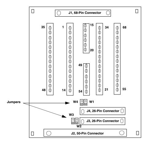
Figure 7: STP268-EC Screw Terminal Panel
