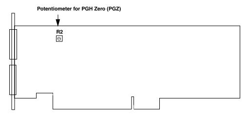
Figure 77: Location of Potentiometer R2 on the DT3016 Board
