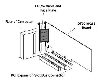
Figure 4: Inserting the DT3010-268 Board in the Computer
