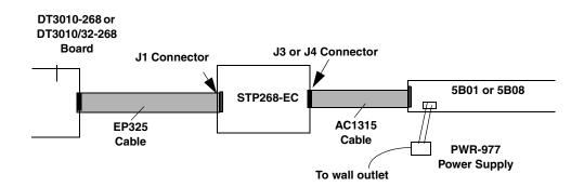
Figure 9: Connecting the 5B Series Backplane to the STP268-EC Screw Terminal Panel
