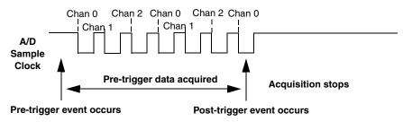
Figure 59: Continuous Pre-Trigger Mode
