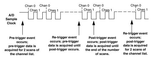
Figure 62: Continuous About-Trigger Mode with Triggered Scan
