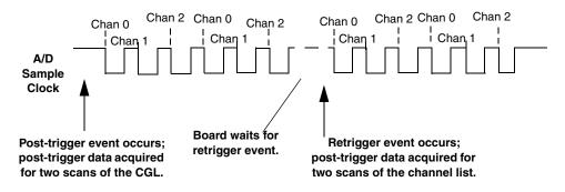
Figure 58: Continuous Post-Trigger Mode with Triggered Scan
