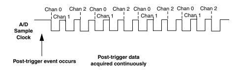
Figure 57: Continuous Post-Trigger Mode without Triggered Scan
