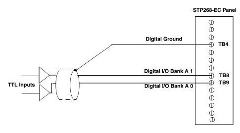
Figure 30: Connecting Digital Inputs to the STP268-EC (Shown for Lines 0 and 1, Bank A)
