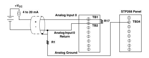
Use current shunt resistor R17 to convert current to voltage;  $250 \Omega$  for 4 to 20 mA = 1 to 5 V. The common side of the external loop supply must either connect to analog ground or, if needed, to a bias return resistor (R1 in this case).
