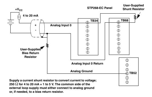
Figure 24: Connecting Current Inputs to the STP268-EC (Shown for Channel 0)
