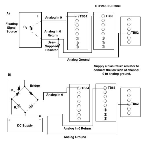
Figure 19: Connecting Differential Voltage Inputs to the STP268-EC (Shown for Channel 0)
