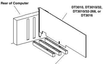
PCI Expansion Slot Bus Connector
