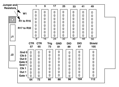
Figure 12: Layout of the DT740 Screw Terminal Panel
