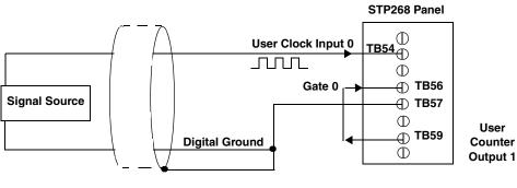
Note that the signals shown for the STP268 screw terminal panel correspond to connector J1.
