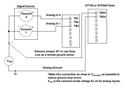
Note that the signals shown for the STP268 screw terminal panel correspond to connector J1.
