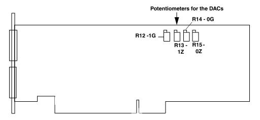
Figure 78: Location of Potentiometers R12 to R15 on the DT3010, DT3010-268, DT3010/32, and DT3010/32-268
