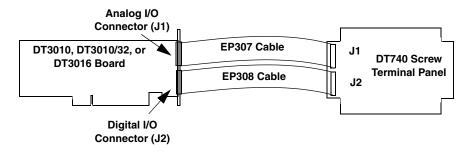
Figure 5: Attaching the DT740 Screw Terminal Panel to the DT3010, DT3010/32, or DT3016 Board
