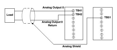
Figure 25: Connecting Analog Output Voltages to the DT740 (Shown for Channel 0)
