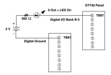
Figure 31: Connecting Digital Outputs to the DT740 (Shown for Line 0, Bank B)
