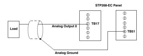
Figure 27: Connecting Analog Output Voltages to the STP268-EC (Shown for Channel 0)
