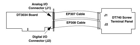
Figure 3: Attaching the DT740 Screw Terminal Panel to the DT3034 Board
