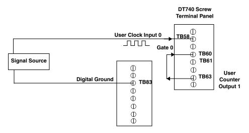
Figure 32: Connecting Frequency Measurement Signals (Shown for Clock Input 0 and External Gate 0)
