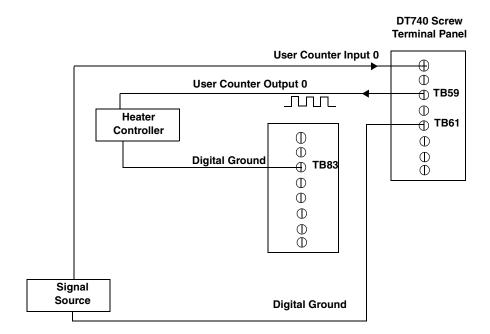
Figure 34: Connecting Rate Generation Signals (Shown for Counter Output 0; a Software Gate is Used)
