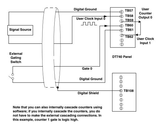
Figure 18: Cascading Counters to the DT740 (Shown for Rate Generation Using Counters 0 and 1 and External Gate 0)
