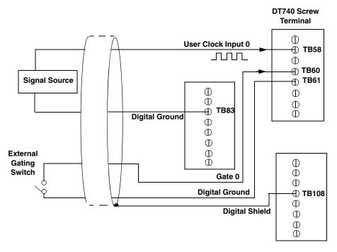
Figure 30: Connecting Event Counting Signals (Shown for Clock Input 0 and External Gate 0)
