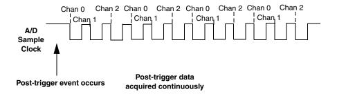
Figure 22: Continuous Post-Trigger Mode without Triggered Scan
