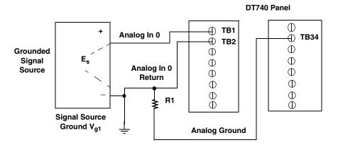
Resistor R1 should be installed for bias return in case the external ground is floating.
