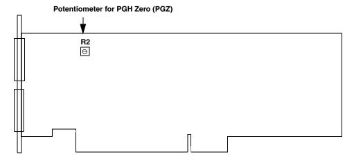
Figure 40: Location of Potentiometer R2 on the DT3034 Board
