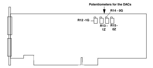
Figure 41: Location of Potentiometers R12 to R15 on the DT3034 Board
