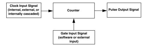
Figure 28: Counter/Timer Channel
