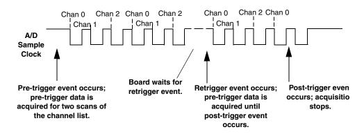
Figure 25: Continuous Pre-Trigger Mode with Triggered Scan
