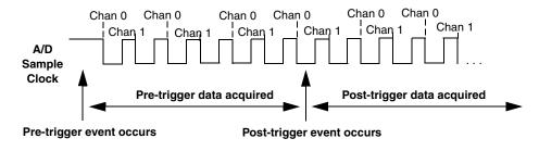
Figure 26: Continuous About-Trigger Mode
