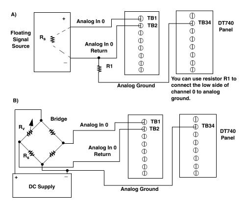
Figure 7: Connecting Differential Voltage Inputs to the DT740 (Shown for Channel 0)
