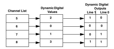
Figure 21: An Example Using Dynamic Digital Outputs
