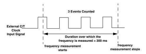
Figure 33: Example of Frequency Measurement
