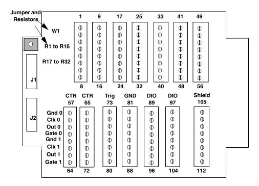
Figure 4: Layout of the DT740 Screw Terminal Panel
