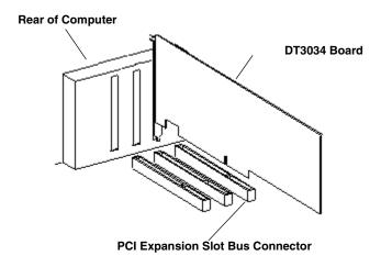
Figure 2: Inserting the DT3034 Board in the Computer
