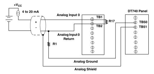
Use current shunt resistor R17 to convert current to voltage; 250  $\Omega$  for 4 to 20 mA = 1 to 5 V. The common side of the external loop supply must either connect to analog ground or, if needed, to a bias return resistor (R1 in this case).
