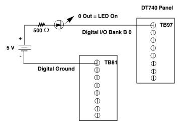
Figure 12: Connecting Digital Outputs to the DT740 (Shown for Line 0, Bank B)
