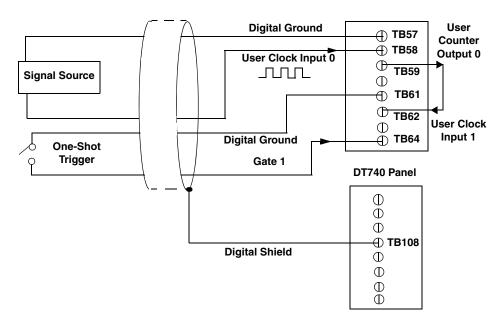
Figure 19: Cascading Counters for the DT740 (Shown for One-Shot Using Counters 0 and 1 and External Gate 1)
