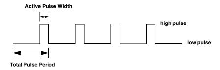
Figure 29: Example of a Low-to-High Pulse Output Type
