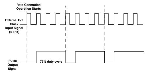
Figure 35: Example of Rate Generation Mode with a 75% Duty Cycle
