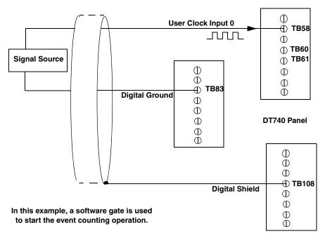
Figure 14: Connecting Event Counting Applications to the DT740 (Shown for Clock Input 0 without an External Gate)
