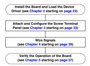
Figure 1: Getting Started Flow Diagram
