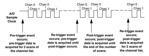
Figure 27: Continuous About-Trigger Mode with Triggered Scan
