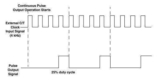
Figure 36: Example of Rate Generation Mode with a 25% Duty Cycle
