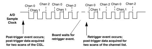
Figure 23: Continuous Post-Trigger Mode with Triggered Scan
