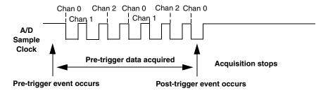
Figure 24: Continuous Pre-Trigger Mode
