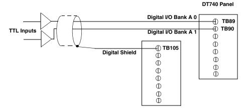
Figure 11: Connecting Digital Inputs to the DT740 (Shown for Lines 0 and 1, Bank A)
