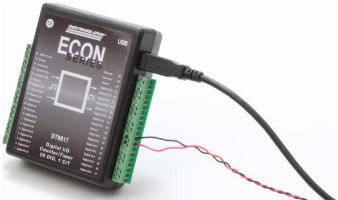
**Figure 5: Wiring to the Screw Terminals of a Module**
