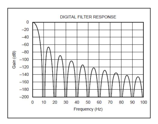
Figure 22: Digital Filter Response (10 Hz Multiples)
