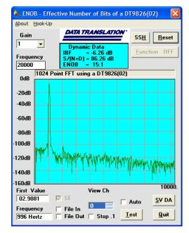
Figure 27A. ENOB of 14.8 bits when measuring a ±5 V, 1 kHz signal with a 40 kHz sample frequency
