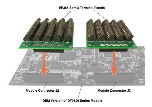
Figure 36: Connecting EP355 Panels to Connector J2 and Connector J3 on the OEM Version of a DT9826 Series Module
