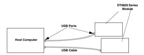
Figure 3: Attaching the Module to the Host Computer
