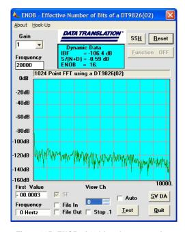
Figure 26B. ENOB of 16 bits when measuring a 0 V signal with a 20 kHz sample frequency
