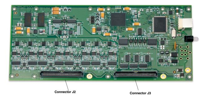
Figure 32: Connectors on OEM Version of DT9826 Series Module
