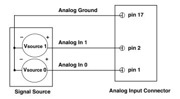
Note: The input impedance of the DT9826 Series is 10 M $\Omega$  (Series 2 k $\Omega$  ,1000 pf Filter)
