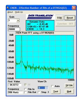
Figure 28A. ENOB of 14.1 bits when measuring a  $\pm 10$  V, 1 kHz sine wave with a 40 kHz sample frequency
