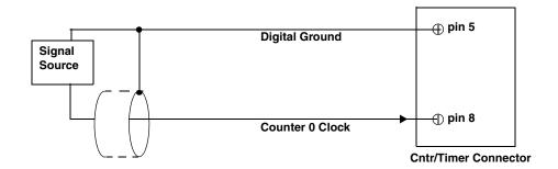
Figure 12: Connecting Counter/Timer Signals to the BNC Connection Box for an Event Counting Operation Without Using a Gate
