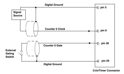
Figure 11: Connecting Counter/Timer Signals to the BNC Connection Box for an Event Counting
