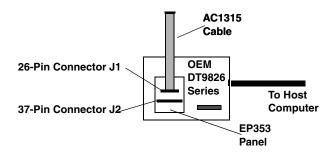
Figure 34: Connecting the AC1315 Cable to the EP353 Panel
