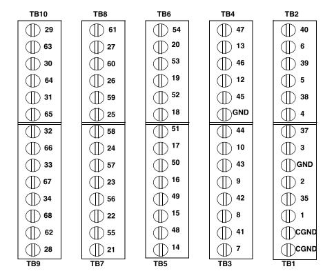
Figure 37: EP355 Screw Terminal Blocks
