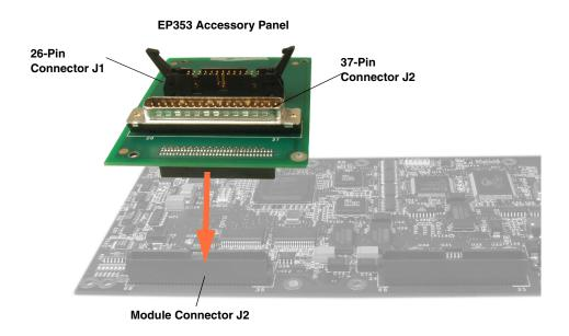
Figure 33: Connecting the EP353 Accessory Panel to Connector J2 on the OEM Version of a DT9826 Series Module
