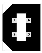
Figure 29: Layout of the USB Connector
