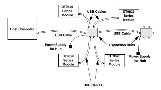
Figure 4: Attaching Multiple Modules Using Expansion Hubs
