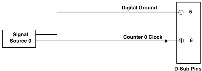
**Figure 18: Connecting Counter/Timer Signals to the D-Sub Pins for a Continuous Edge-to-Edge Measurement Operation**
