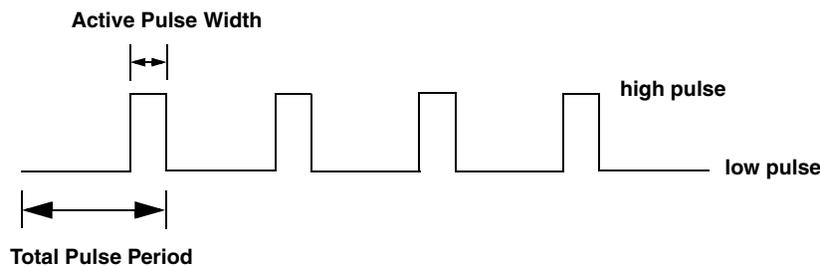
**Figure 24: Example of a Low-to-High Pulse Output Type**
