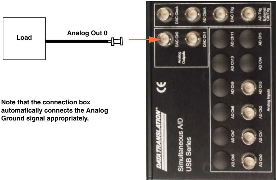
Note that the connection box automatically connects the Analog Ground signal appropriately.
