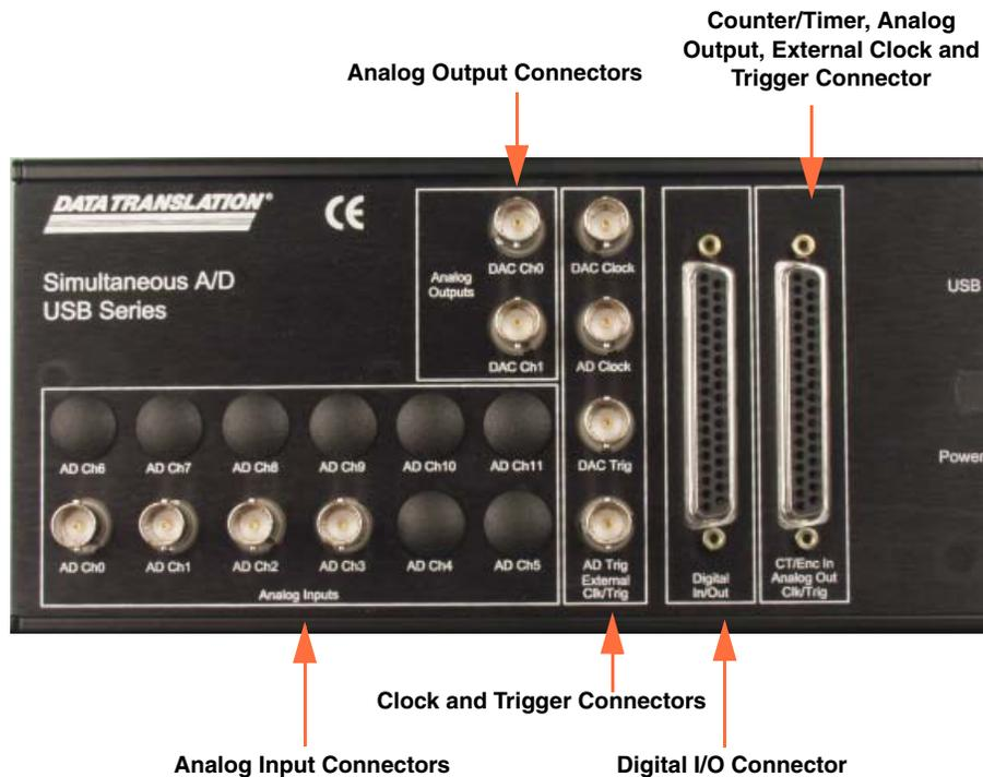
**Figure 7: DT9832-04-2-BNC Version of the BNC Connection Box**
