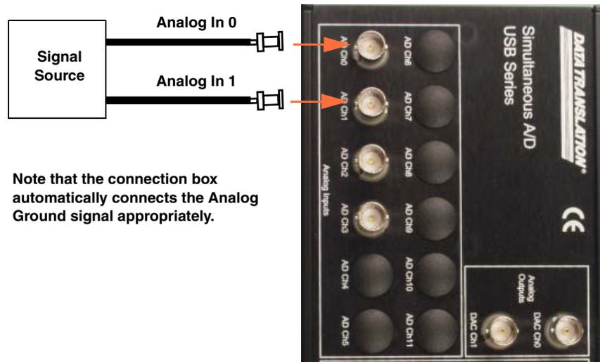
Figure 8: Connecting Single-Ended Inputs to the BNC Connection Box
