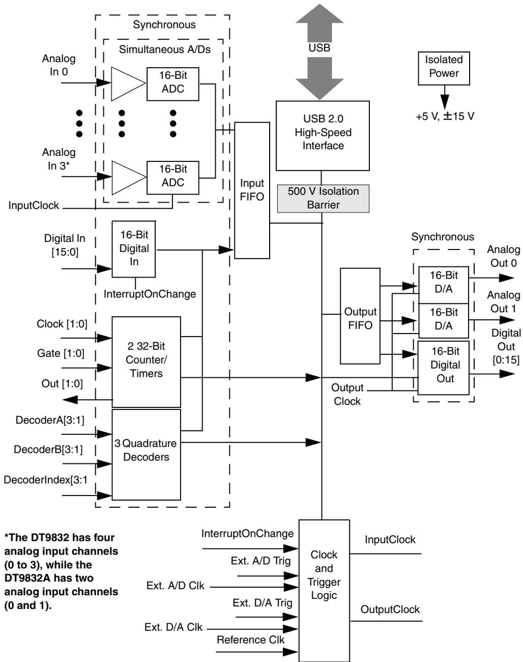
Figure 21: Block Diagram of the DT9832 Series Modules
