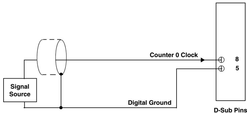
**Figure 16: Connecting Counter/Timer Signals to the D-Sub Pins for a Period/Pulse Width Measurement Operation**
