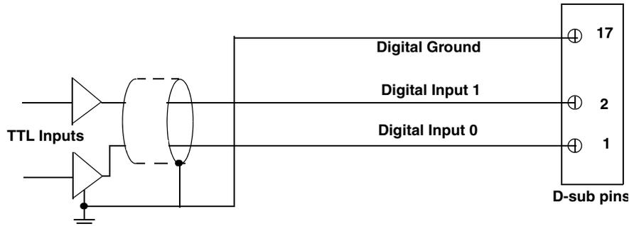
Figure 10: Connecting Digital Inputs to the D-Sub Pins
