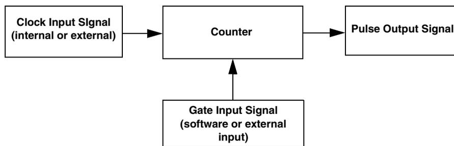
**Figure 23: Counter/Timer Channel**
