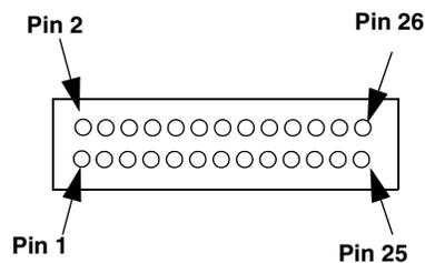
**Figure 30: Orientation of the Pins for Connectors J1 on the EP353 Panel**
