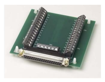
Figure 4: STP37 Screw Terminal Panel
