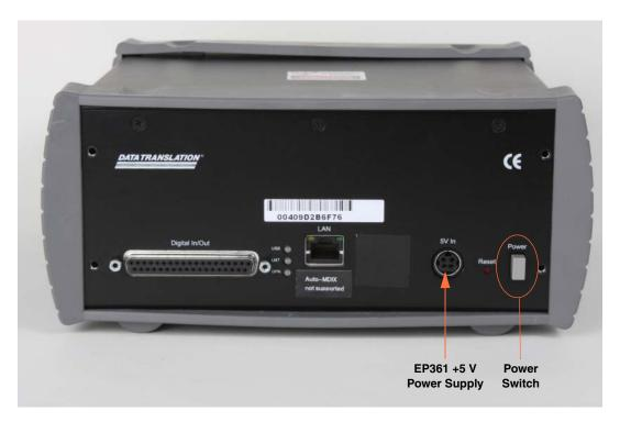
Figure 12: Attaching a +5 V Power Supply to the Instrument
