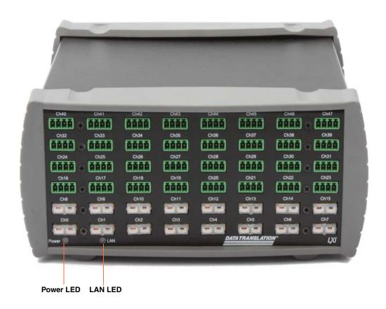
Figure 13: LEDs on the Front Panel of the Instrument
