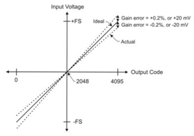
Figure 13. ADC Transfer function with gain error
