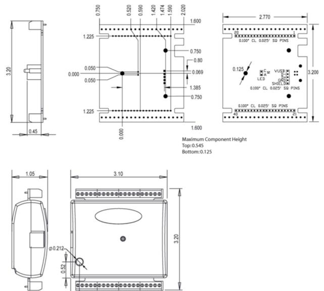
Figure 15. Circuit board (top) and enclosure dimensions
