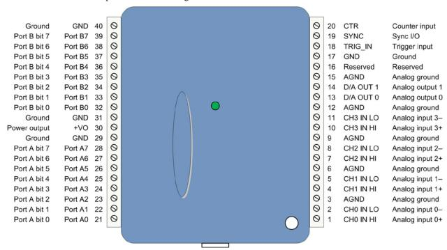
Figure 4. Differential mode pinout
