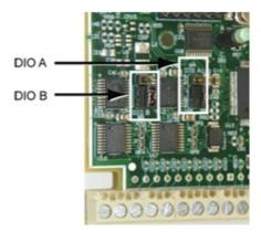
Figure 9. Pull-up/down jumper locations
