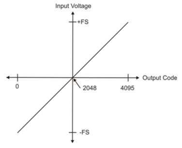
Figure 11. Ideal ADC transfer function
