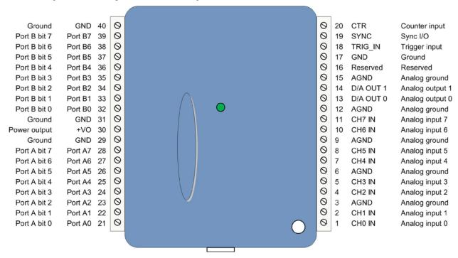
Figure 3. Single-ended mode pinout
