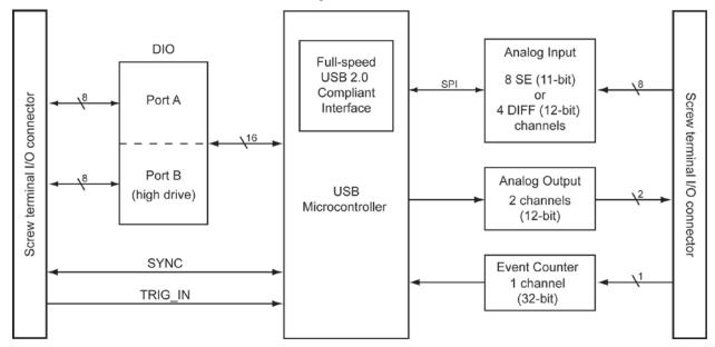
Figure 1. USB-1208FS-Plus functional block diagram
