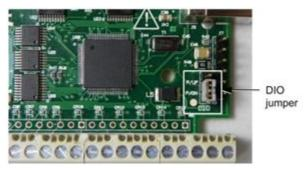
Figure 5. Pull-up/down jumper location
