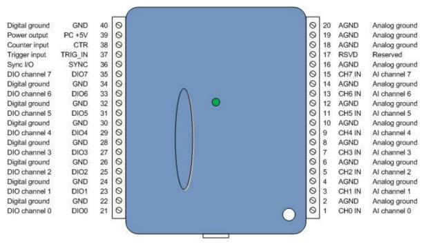
Figure 3. Screw terminal pinout
