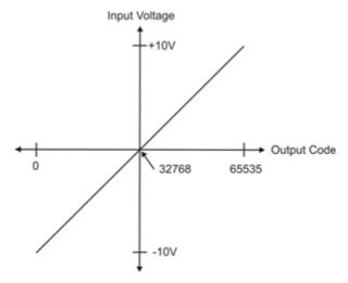
Figure 7. Ideal ADC transfer function
