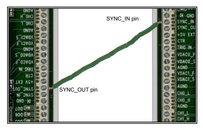
Figure 10. Configuring for synchronous data acquisition
