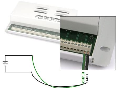
Figure 6. Single-ended measurement connection
