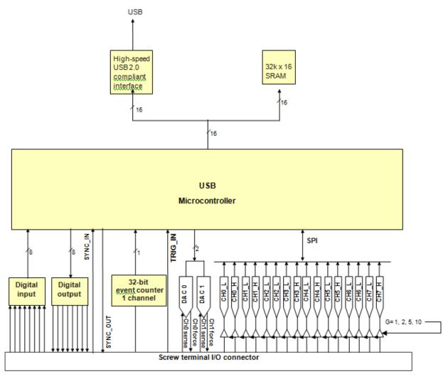
Figure 2. USB-1608HS-2AO functional block diagram
