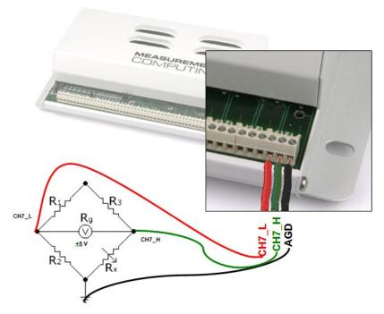
Figure 7. Differential measurement connection
