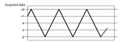
Figure 11. Trigger above, level-sensitive
