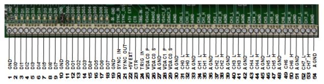
Figure 4. USB-1608HS-2AO screw terminal functions
