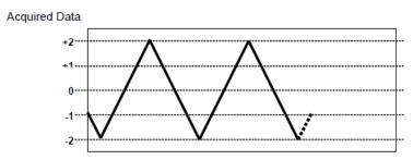
Figure 12. Trigger below, level-sensitive
