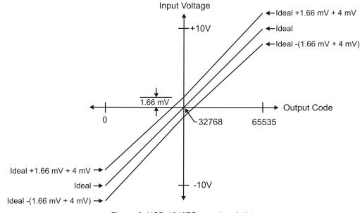
Figure 8. USB-1616FS error band plot
