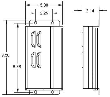
Figure 10. USB-1616FS enclosure dimensions
