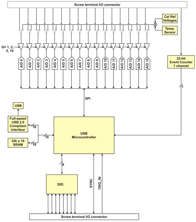
Figure 1. USB-1616FS functional block diagram
