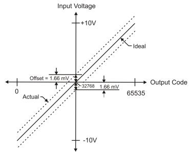
Figure 6. USB-1616FS transfer function with offset error
