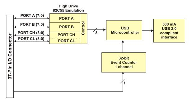
Figure 1. USB-DIO24H/37 functional block diagram
