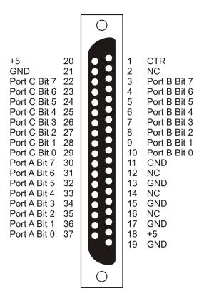
Figure 2. I/O connector pinout
