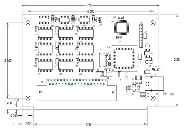
Figure 6. Circuit board dimensions
