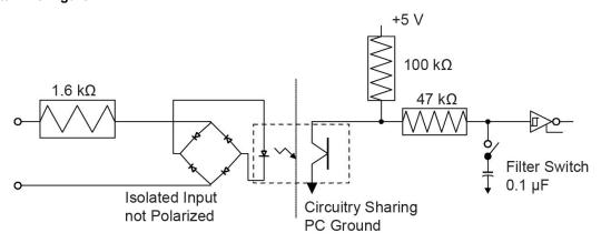
Figure 5. USB-PDISO8 single-channel configuration
