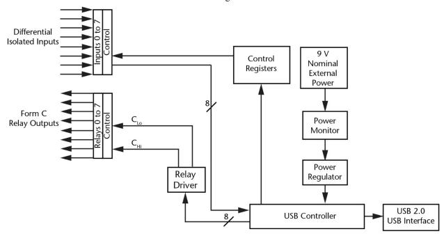
Figure 1. USB-PDISO8 functional block diagram
