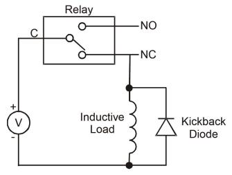
Figure 8. Relay contact protection circuit
