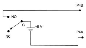
Figure 6. Schematic of battery-to-relay connection
