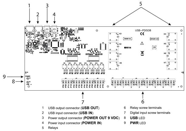
Figure 2. USB-PDISO8 components
