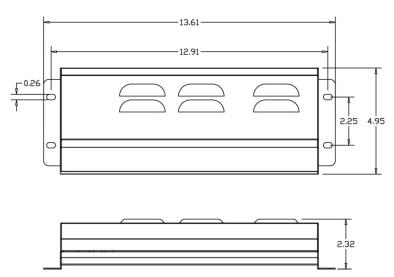
Figure 9. Circuit board (top) and housing dimensions
