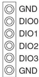
Figure 4. Screw terminal pinout.
