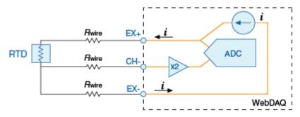
Figure 10. 3-wire RTD circuitry
