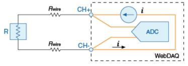
Figure 11. 2-wire Resistance and quarter-bridge circuitry
