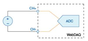
Figure 6. Voltage circuitry
