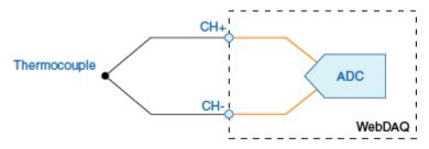
Figure 8. Thermocouple circuitry
