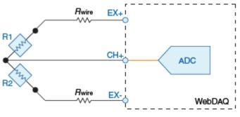
Figure 13. Half-bridge circuitry
