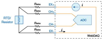
Figure 9. 4-wire resistance and RTD circuitry
