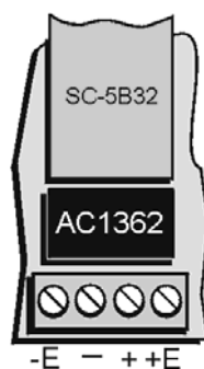
AC1362 Current Sense Resistor Install Location
