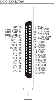
Figure 2-1. Main connector pinout
