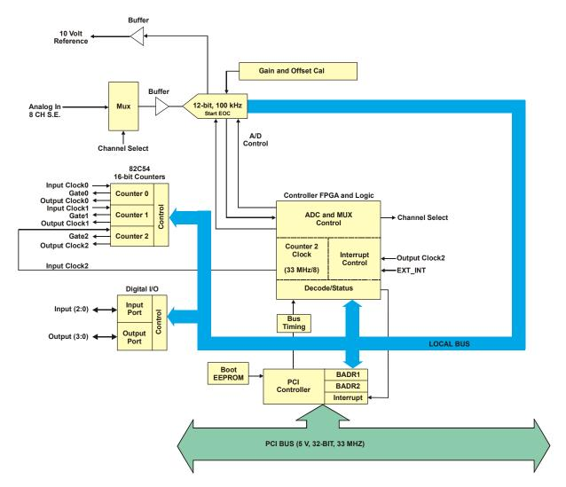
Figure 1-1. PCI-DAS08 block diagram
