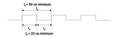
Figure 22. D/A EXTERNAL TIME BASE signal timing
