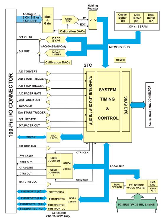
Figure 4. Block diagram – PCI-DAS6025 and PCI-DAS6023
