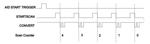
Figure 6. Data Acquisition Example for Conventional Triggering
