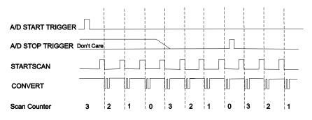
Figure 9. Pre-triggered data acquisition example
