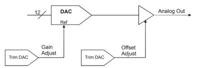
Figure 30. Analog output calibration
