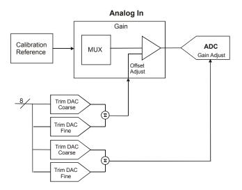
Figure 29. Analog input calibration
