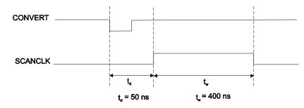
Figure 5. SCANCLK Signal Timing
