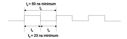
Figure 16. A/D EXTERNAL TIME BASE signal timing
