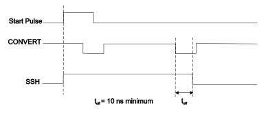
Figure 13. SSH signal timing
