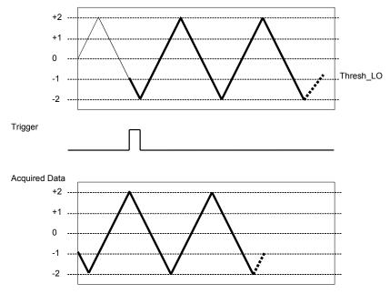
Figure 20. Trigger negative slope
