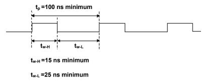
Figure 32. CTR1 CLK signal timing
