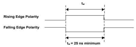
Figure 33. CTR1 GATE signal timing
