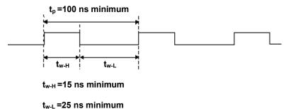
Figure 35. CTR2 CLK signal timing
