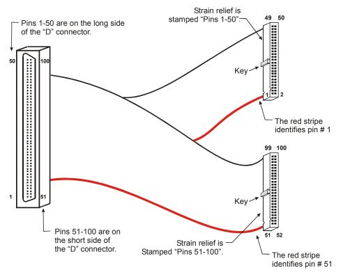
Figure 1. C100HD50-x cable connections
