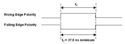
Figure 7. A/D START TRIGGER input signal timing
