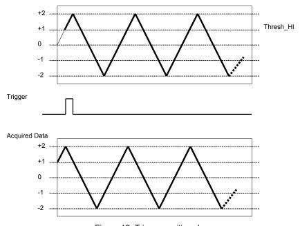
Figure 19. Trigger positive slope
