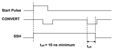
Figure 13. SSH signal timing
