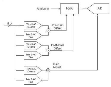
Figure 38. Analog input calibration - basic elements
