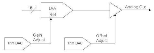
Figure 39. Analog output calibration - basic elements
