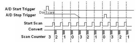
Figure 9. Pre-triggered data acquisition example
