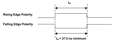
Figure 27. D/A START TRIGGER input signal timing
