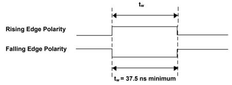
Figure 29. D/A CONVERT input signal timing
