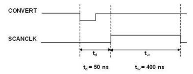
Figure 5. SCANCLK signal timing
