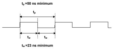
Figure 16. A/D EXTERNAL TIME BASE signal timing
