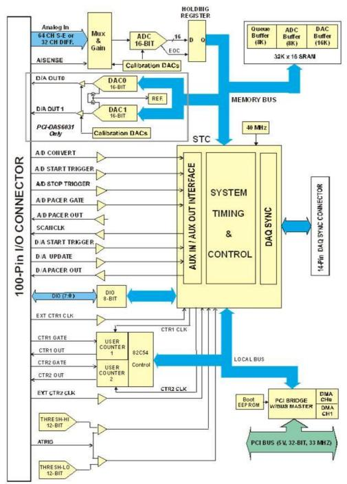
Figure 4. Block diagram – PCI-DAS6031 and PCI-DAS6033
