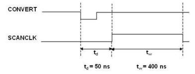
Figure 5. SCANCLK signal timing
