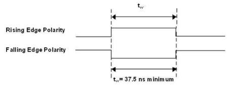
Figure 10. A/D STOP TRIGGER input signal timing
