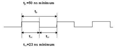
Figure 30. D/A EXTERNAL TIME BASE signal timing
