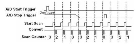
Figure 9. Pre-triggered data acquisition example
