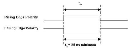
Figure 35. CTR2 GATE signal timing
