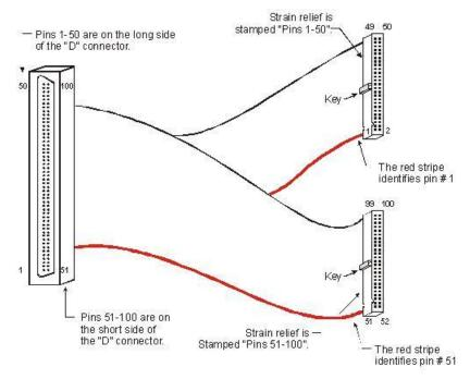
Figure 1. C100HD50-x Cable Connections
