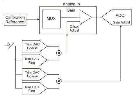
Figure 37. Analog input calibration - basic elements
