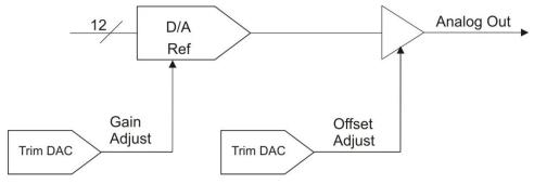
Figure 38. Analog output calibration - elements
