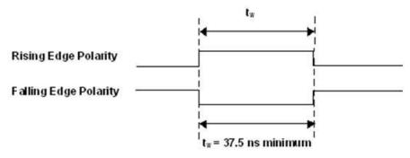
Figure 28. D/A CONVERT input signal timing
