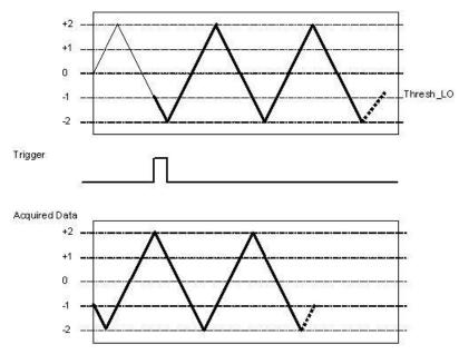
Figure 19. Trigger Negative Slope
