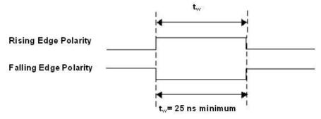
Figure 32. CTR1 GATE signal timing
