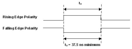
Figure 26. D/A START TRIGGER input signal timing
