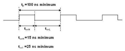
Figure 31. CTR1 CLK signal timing
