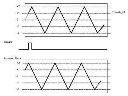
Figure 18. Trigger Positive Slope
