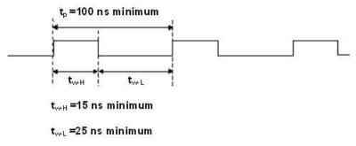
Figure 34. CTR2 CLK signal timing
