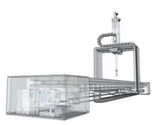
The Probe Permeameter machine makes measurements in core samples using an X-Y control system with under one millimeter precision. A Raspberry Pi 4 board is at the heart of the solution, providing enough processing power for the machine vision and data acquisition and control functions.
