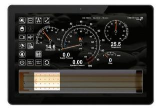
Data is sent via WiFi to a remote touch screen interface where the operator can view gas pressure, temperature, and flow data in real time.
