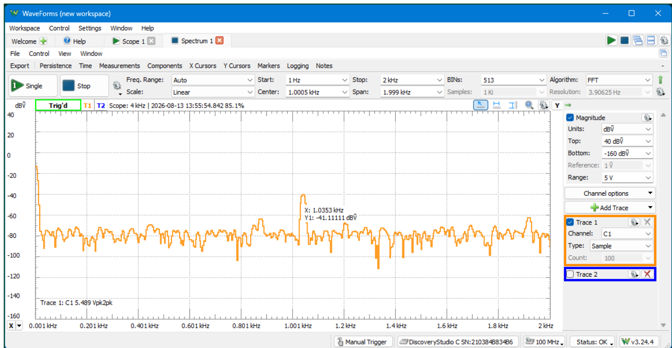
Figure 7. Frequency Spectrum of the Microphone Output Signal
