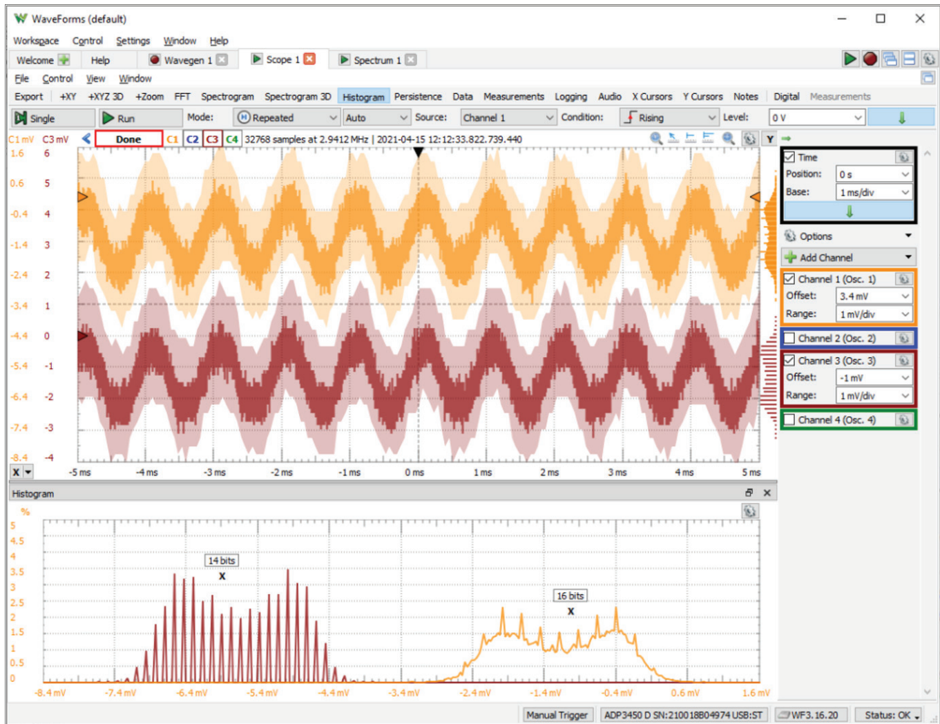
Figure 2: Histogram of 14-bit resolution oscilloscope and 16-bit resolution oscilloscope.
