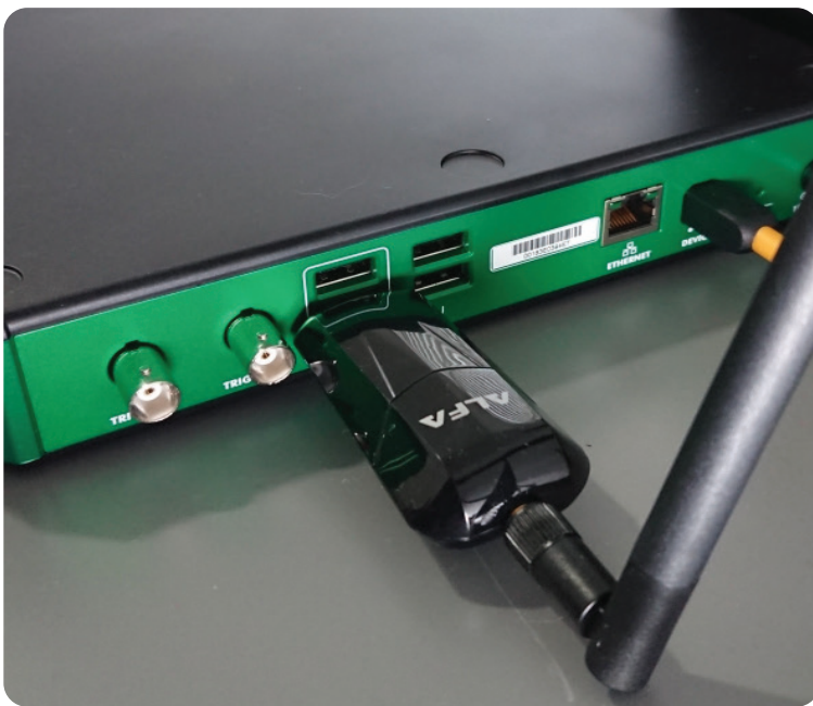
Figure 4: A USB Wi-Fi dongle connected in the back of the ADP3450 for remote testing and control.
