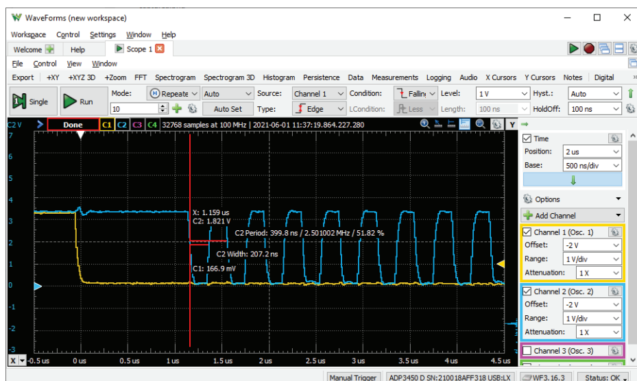
Figure 4: Measuring a 2.5 MHz SPI clock's frequency with a pulse measurement tool.
